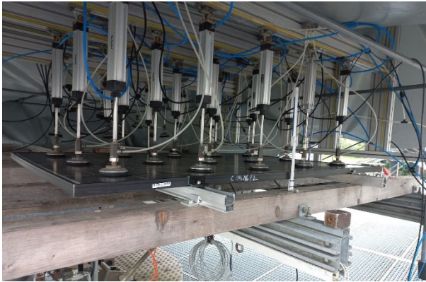
Figure 10: Collector under positive load test of 2400 Pa
