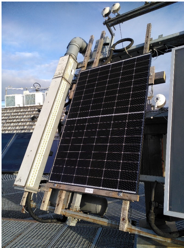
Figure 6: Collector installed on the SPF solar simulator
