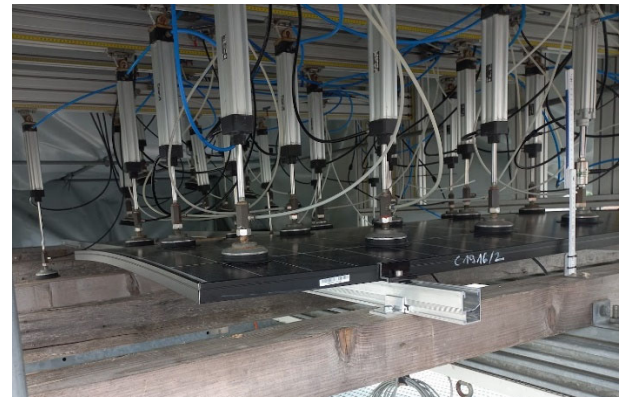
Figure 11: Collector under negative load test of 2400 Pa
