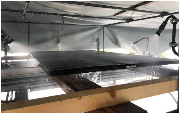
Figure 12: Collector in rain test
