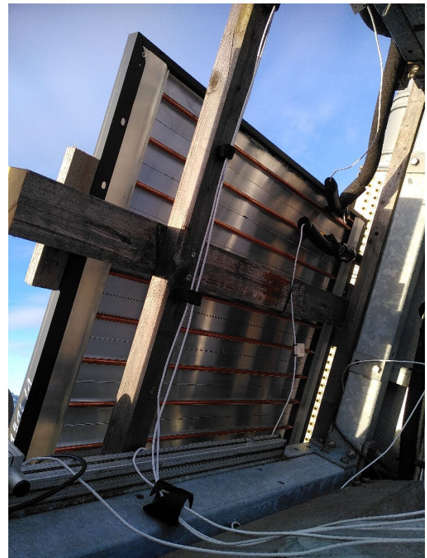
Figure 7: Collector installed on the SPF outdoor test rig
